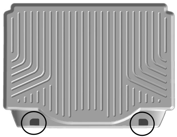
TO ACCESS THE FACTORY CARPET TIE-DOWN LOCATIONS AT THE REAR OF YOUR VEHICLE SIMPLY TRIM THE MATERIAL FROM THE TWO LOWERED AREAS CORRESPONDING TO THE TIE-DOWN LOCATIONS. THESE AREAS ARE SHOWN ABOVE DARKENED AND CIRLCED.
