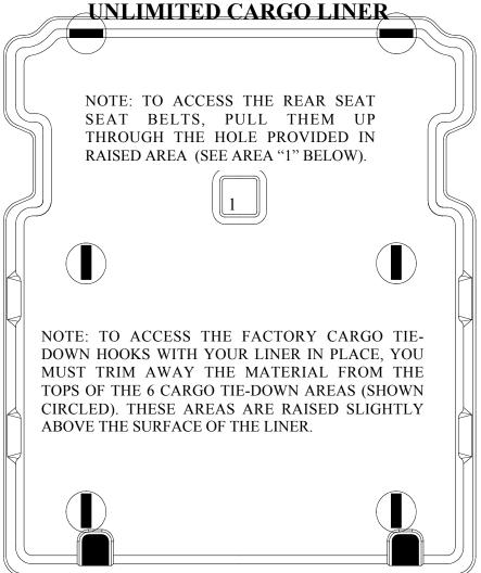
TO ACCESS THE FACTORY CHILD SEAT SAFETY RESTRAINT ANCHORS, TRIM AWAY THE MATERIAL FROM THE TOPS OF THE TWO (2) RAISED AREAS (SHOWN ABOVE DARKENED).
