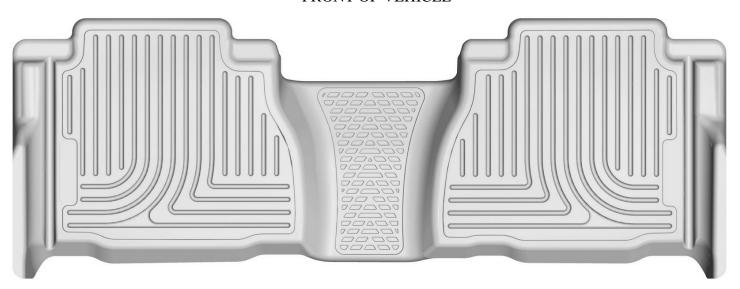
TO EASE INSTALLATION OF YOUR TUNDRA SECOND SEAT LINER, MOVE THE FRONT SEATS TO THEIR MOST FORWARD POSITIONS AND FOLD UP (DOUBLE CAB) OR SLIDE BACK (CREWMAX) THE SECOND ROW SEATS. WITH THIS DONE, INSERT THE LINER IN VEHICLE ANGLING THEM SO THAT THE FRONT EDGE OF THE LINER IS SEATED INTO PLACE FIRST, THEN, LOWERING THE REAR EDGE. ONCE THE LINER IS INSTALLED, REPOSITION THE FRONT SEATS AS DESIRED.
