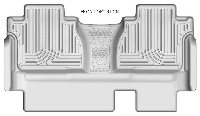
TO EASE INSTALLATION OF YOUR DOUBLE CAB TRUCK 2<sup>ND</sup> SECOND SEAT LINER, MOVE THE FRONT ROW SEATS TO THEIR MOST FORWARD POSITIONS AND FLIP UP THE 2<sup>ND</sup> ROW SEAT BOTTOMS. WITH THIS DONE, INSTALL YOUR LINER AS SHOWN ABOVE. ONCE THE LINER IS INSTALLED, REPOSITION THE FRONT SEATS AS DESIRED.
