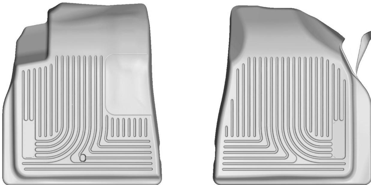
DEPENDING ON THE FACTORY OPTIONS INSTALLED ON YOUR VEHICLE, YOUR PASSENGER'S SIDE LINER MAY REQUIRE TRIMMING. TO DETERMINE IF TRIMMING MIGHT BE NEEDED, INSTALL THE PASSENGER SIDE LINER AND OBSERVE THE PORTION OF THE LINER THAT MATCHES UP TO THE UPPER RIGHT HAND KICK PANEL. IF THE LINER APPEARS TOO WIDE AND DOES NOT LIE FLAT, YOU WILL NEED TO TRIM YOUR LINER. IF THE LINER CONTOURS THE AREA CORRECTLY, NO TRIMMING IS NEEDED (SEE PHOTOS OF INSTALLED PARTS ON BACK OF PAGE).
