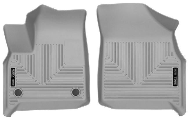
TO EASE INSTALLATION OF YOUR FRONT FLOOR LINERS, FIRST SLIDE BOTH FRONT ROW SEATS COMPLETELY BACK TO EXPOSE THE MAXIMUM AMOUNT OF THE FLOORING. NOTE THAT THE FRONT DRIVER'S SIDE LINER ATTACHES TO THE FACTORY MAT RETAINING POSTS. TAKE CARE THAT THE LINER IS SECURELY POSITIONED ON THE FACTORY POSTS WHEN INSTALLED. ONCE LINERS ARE IN PLACE, REPOSITION THE FRONT SEATS AS DESIRED.
