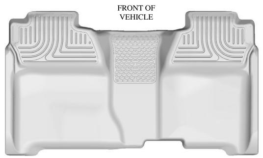
TO EASE INSTALLATION OF YOUR SILVERADO/SIERRA CREW CAB TRUCK SECOND SEAT LINER, MOVE BOTH FRONT ROW SEATS TO THEIR MOST FORWARD POSITION AND FLIP UP THE 2<sup>ND</sup> ROW SEATS. WITH THIS DONE, INSTALL YOUR LINER, POSITIONING IT AS SHOWN IN THE IMAGE ABOVE. ONCE THE LINER IS INSTALLED, REPOSITION THE FRONT SEATS AS DESIRED AND LOWER YOUR 2<sup>ND</sup> ROW SEATS.
