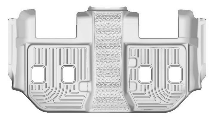
BEFORE ATTEMPTING TO INSTALL YOUR LINER, FIRST FLIP/FOLD YOUR SECOND ROW BUCKET SEATS FORWARD TO EXPOSE THE 3<sup>RD</sup> ROW FLOOR PAN. WITH THIS DONE YOU CAN POSITION THE LINER IN THE FLOOR ORIENTED AS SHOWN ABOVE. THE "TONGUE" AREA PROVIDES COVERAGE BETWEEN THE 2<sup>ND</sup> ROW BUCKET SEATS AND TUCKS UNDER THE REAR EDGE OF YOUR 2<sup>ND</sup> SEAT LINER.
