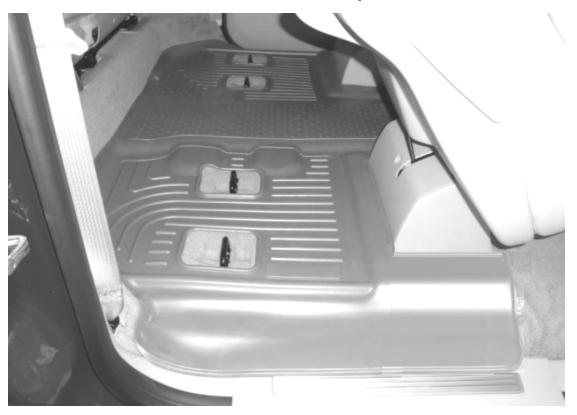
NOTE SEAT ATTACHES TO FLOOR THROUGH LINER
