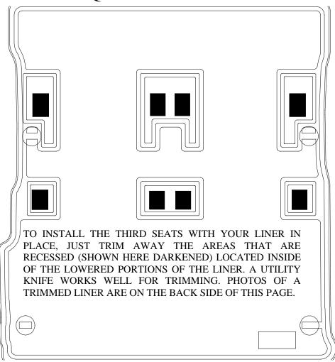
TO ACCESS THE FACTORY CARGO HOOK TIE DOWN LOCATIONS WITH YOUR CARGO LINER IN PLACE YOU MUST FIRST MAKE A SLIT IN THE FOUR (4) RAISED AREAS ON YOUR LINER (SHOWN CIRCLED). THEN, PUSH THE HOOK RINGS UP THROUGH THE LINER.
