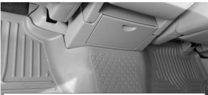
THIS IMAGE SHOWS PART #1919 INSTALLED IN A TRUCK WITH A FRONT ROW BENCH SEATING AND THE REAR FACING CUPHOLDER. THE LINER HAS BEEN TRIMMED ALONG THE MOLDED IN GROOVE. THE CUP HOLDER IS FULLY FUNCTIONAL. A UTILITY KNIFE OR HEAVY SHEARS WORK WELL FOR TRIMMING.
