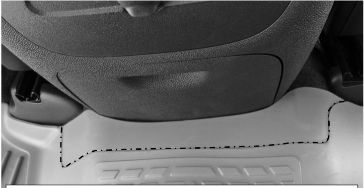
THIS IMAGE SHOWS PART #1919 INSTALLED IN A TRUCK WITH A FRONT ROW CONSOLE. NO TRIMMING IS NEEDED FOR TRUCKS WITH THIS FEATURE. THE IMAGE SHOWS THE TRIM GROOVE (HIGHLIGHTED BY THE DASHED LINE) USED WHEN TRIMMING FOR MODELS WITH FRONT ROW BENCH SEATING AND THE REAR FACING CUPHOLDER.
