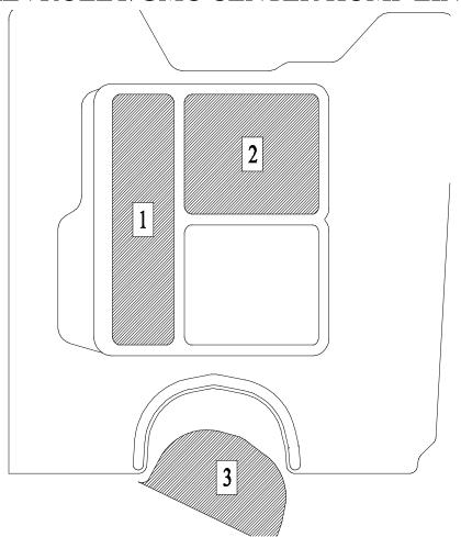
NOTE: IF YOUR VEHICLE IS EQUIPPED WITH A MANUAL TRANSFER CASE, REMOVE THE TREAD PLATE FROM AREA "1" SHOWN ABOVE. IF IT IS EQUIPPED WITH A MANUAL TRANSMISSION, REMOVE THE TREAD PLATE FROM AREA "2" SHOWN ABOVE. IF IT IS EQUIPPED WITH A CENTER CONSOLE, TRIM AWAY AREA "3" SHOWN ABOVE. A UTILITY KNIFE OR HEAVY SCISSORS WORK WELL FOR TRIMMING.
