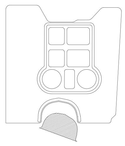
NOTE: IF YOUR VEHICLE IS EQUIPPED WITH A CENTER CONSOLE, IT WILL BE NECESSARY TO TRIM YOUR LINER AS SHOWN ABOVE. THE NECESSARY TRIMMING IS EASILY DONE BY REMOVING THE SHADED SECTION SHOWN ABOVE. USING A UTILITY KNIFE OR HEAVY SCISSORS, REMOVING THE MATERIAL INSIDE OF THE OUTLINING RAISED BAND.
