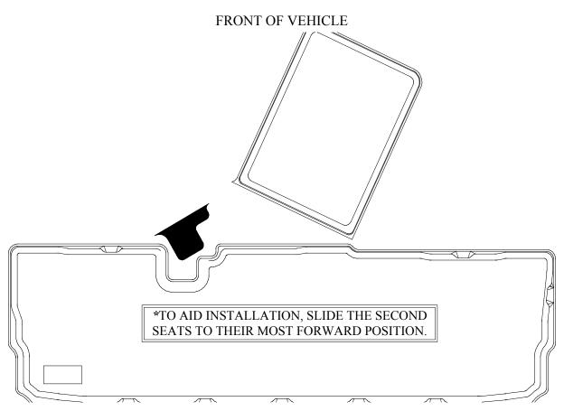
EXCURSION OWNERS WITHOUT SECOND ROW CAPTAIN'S CHAIRS WILL NEED TO TRIM AWAY THE AREA SHOWN DARKENED BELOW. A TRIM GROOVE IS MOLDED IN TO USE AS A GUIDE. THE "TONGUE" SHOWN TRIMMED CAN ALSO BE REMOVED OR TUCKED UNDER THE SECOND ROW BENCH SEAT. TRIMMING PHOTOS ARE INCLUDED ON THE BACK OF THIS PAGE.
