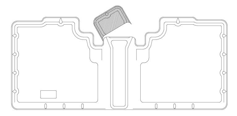
IF YOUR TRUCK IS EQUIPPED WITH A CENTER CONSOLE YOU WILL NEED TO TRIM YOUR HUSKY LINER, REMOVING THE AREA ABOVE THE HORIZONTAL BAND AS SHOWN ABOVE. FOLLOW THE TRIM LINE ETCHED ON THE PART. A UTILITY KNIFE OR HEAVY SHEARS WORK WELL FOR TRIMMING.
