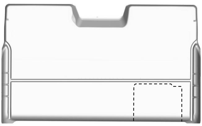
IF YOUR VEHICLE IS EQUIPPED WITH A FACTORY SUBWOOFER LOCATED UNDER THE PASSENGER'S SIDE REAR SEAT, YOU WILL NEED TO TRIM YOUR LINER TO ACCOMMODATE THIS FEATURE. TO TRIM THE LINER, USE THE STEP FORMED BY THE LOWERED AREA IN YOUR LINERS AS A TRIMMING GUIDE AND THE MATERIAL FROM THE SPACE THE SUBWOOFER OCCUPIES. PHOTOS OF THE TRIMMED PART ARE INCLUDED ON BACK OF THIS PAGE.
