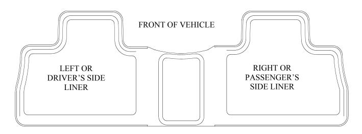
TO EASE INSTALLATION OF LINER, POSITION FRONT SEATS TO THEIR MOST FORWARD POSITIONS. ONCE LINER IS INSTALLED, REPOSITION SEATS AS DESIRED.
