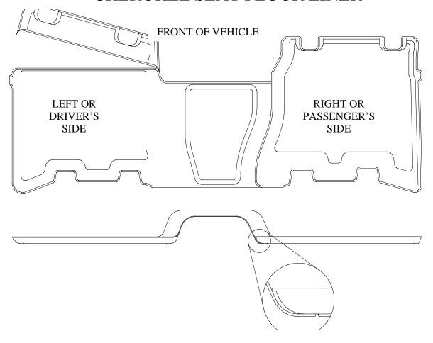
JEEP OWNERS WITH POWER SEATS MAY NEED TO TRIM THEIR DRIVER'S SIDE LINER AS SHOWN ABOVE TO ALLOW SUFFICIENT SEAT TRACK CLEARANCE. TRIM ALONG THE MIDDLE OF THE RAISED RIDGE BISECTING THE LINER. A UTILITY KNIFE OR SCISSORS WORK WELL.
