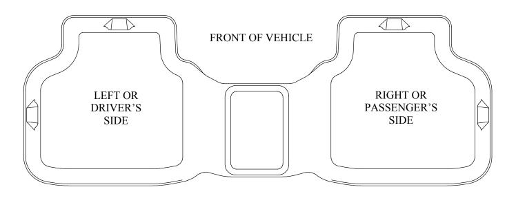
TO EASE INSTALLATION OF YOUR DODGE JOURNEY SECOND SEAT LINER, MOVE BOTH FRONT SEATS TO THEIR MOST FORWARD POSITION BEFORE INSTALLING LINER. ONCE LINER IS IN PLACE, REPOSITION THE FRONT SEATS AS DESIRED.
