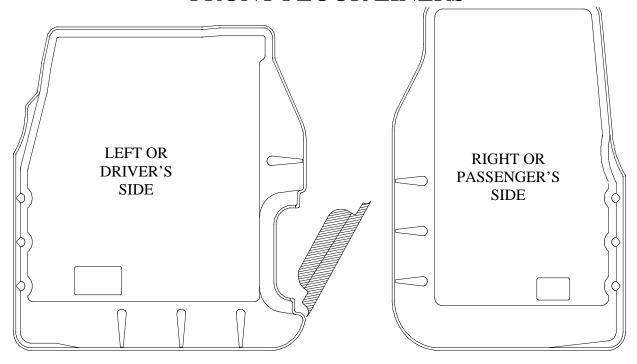
IF YOUR TRUCK IS EQUIPPED WITH A MANUAL TRANSFER CASE SHIFTER, YOU WILL NEED TO TRIM YOUR MAT AS SHOWN ABOVE. TRIM LEAVING A ONE-QUARTER INCH (1/4") LIP ALONG THE FLAT ANGLED SURFACE AND FOLLOWING AROUND THE RAISED SURFACE THAT MAKES THE SLOPING WALL OF THE LINER. A UTILITY KNIFE OR HEAVY SCISSORS WORKS WELL FOR TRIMMING. SEE THE BACK OF THIS INSTRUCTION SHEET FOR A MORE DETAILED VIEW.
