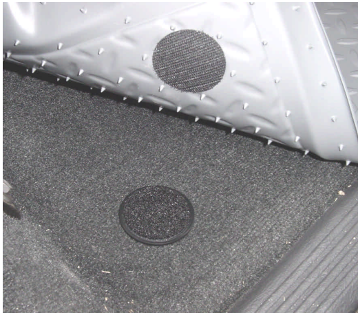
PHOTO 3. ANCHOR SCREW SHOWN INSTALLED IN CARPET ALIGNED BELOW HOOK PAD.
