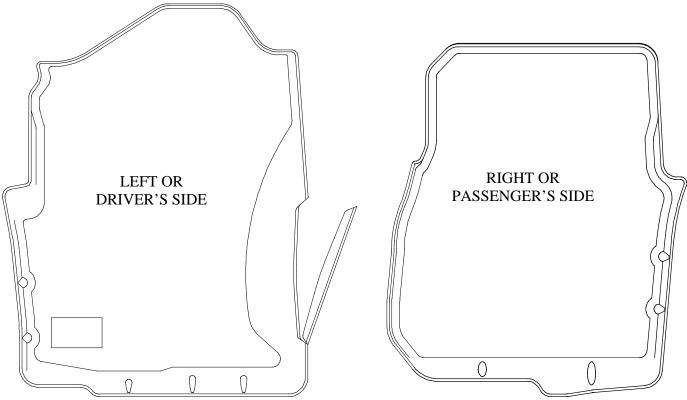
IF YOUR VEHICLE IS EQUIPPED WITH A MANUAL TRANSFER CASE SHIFTER, YOU WILL NEED TO TRIM YOUR LINER AS SHOWN ABOVE. TRIM AWAY THE RAISED AREA ALONG THE WALL OF YOUR LINER. YOUR LINER WILL NOW FIT AROUND THE TRANSFER CASE SHIFTER HOUSING. A UTILITY KNIFE OR HEAVY SCISSORS WORKS WELL FOR TRIMMING YOUR LINER.
