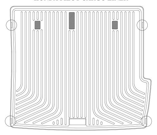
TO ACCESS THE FACTORY CARGO TIE DOWN HOOKS WITH YOUR LINER IN PLACE, TRIM AWAY THE MATERIAL FROM THE RECESSED AREAS ON YOUR LINER THAT CORRESPOND WITH THE HOOKS (SHOWN ABOVE CIRCLED). TO ACCESS THE FACTORY CHILD SEAT SAFETY HOOK LOCATIONS LOCATED IN THE CARGO FLOOR, REMOVE THE MATERIAL FROM THE CORRESPONDING AREA(S) DENOTED WITH A RAISED PERIMETER BAND (SHOWN ABOVE DARKENED). A UTILITY KNIFE WORKS WELL FOR TRIMMING.
