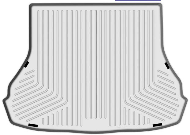
YOUR HYUNDAI ELANTRA TRUNK LINER IS DESIGNED TO ALLOW ACCESS TO THE FACTORY CARGO TIE-DOWN HOOKS. TO ACCESS THE FOUR (4) HOOK LOCATIONS, SIMPLY TRIM AWAY THE MATERIAL FROM THE CORRESPONDING LOWERED AREAS IN THE LINER LOCATED DIRECTLY ABOVE THE HOOK LOCATIONS (SHOWN HERE DARKENED). A UTILITY KNIFE WORKS WELL FOR TRIMMING.
