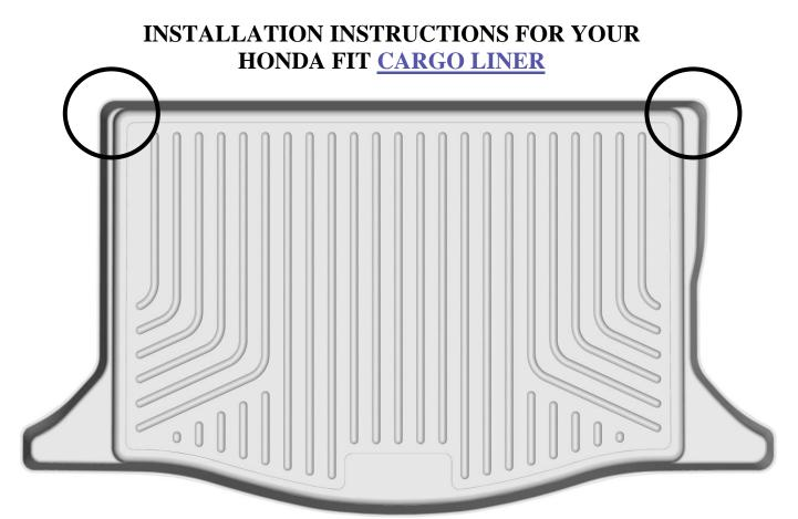
TO MORE EASILY ACCESS THE FACTORY CARGO TIE-DOWN HOOK LOCATIONS WITH YOUR LINER IN PLACE, YOUR LINER HAS TWO TRIM AREAS LOCATED ON THE BACK WALL (SEE CIRCLED AREAS ON DRAWING ABOVE). THE AREAS THAT CAN BE TRIMMED ARE LOWERED IN THE PART AND CAN EASILY BE TRIMMED WITH A UTILITY KNIFE OR HEAVY SHEARS.
