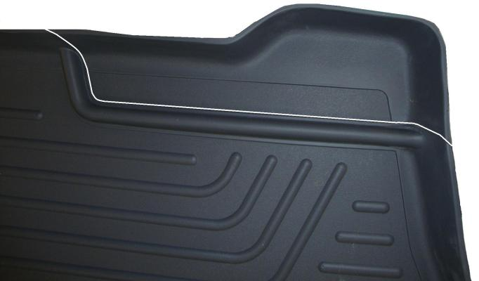
THE LINE THROUGH THE PART IN THE PHOTO ABOVE HIGHLIGHTS THE TRIM NEEDED FOR THE SUBWOOFER ACCOMMODATION. THERE IS A STEP IN THE PART TO GUIDE TRIMMING.
