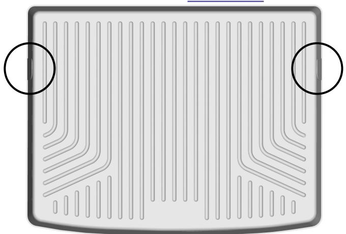
YOUR VOLT CARGO LINER IS DESIGNED TO ALLOW ACCESS TO THE FACTORY CARGO TIE-DOWN HOOKS VIA TRIMMING. TO TRIM, SIMPLY REMOVE THE MATERIAL FROM THE LOWERED AREAS ON EACH SIDE OF THE LINER (AREAS CIRCLED ABOVE). A UTILITY KNIFE OR HEAVY SHEARS WORK WELL FOR TRIMMING.
