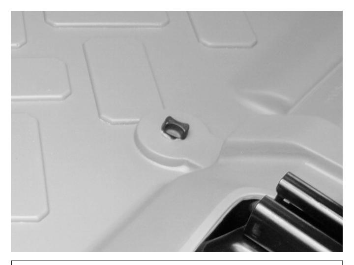
HUSKY LINER PART #3593 SHOWN INSTALLED IN AN FJ CRUISER WITH AUTOMATIC TRANSMISSION. NOTE THAT LINERS MUST BE ATTACHED OVER FACTORY MAT HOOKS TO HELP SECURE LINERS IN POSITION.
