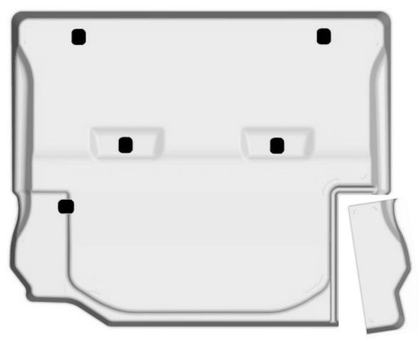
NOTICE: IF YOUR WRANGLER UNLIMITED HAS THE OPTIONAL SUB-WOOFER MOUNTED ON THE PASSENGER SIDE PANEL IN THE CARGO AREA, YOUR LINER WILL NEED TO BE TRIMMED BEFORE INSTALLING. TO TRIM, CUT ALONG THE EDGE OF THE MOLDED STEP THAT RUNS ALONG THE RAISED RIB IN THE PART AS SHOWN ABOVE (ALSO SEE PHOTOS THE BACK OF THIS PAGE). THE DARKENED AREAS ABOVE ARE CARGO TIE-DOWN HOOK LOCATIONS. THESE CAN BE ACCESSED WITH THE LINER IN PLACE BY TRIMMING AWAY THE AREA INSIDE OF THE RAISED BAND.
