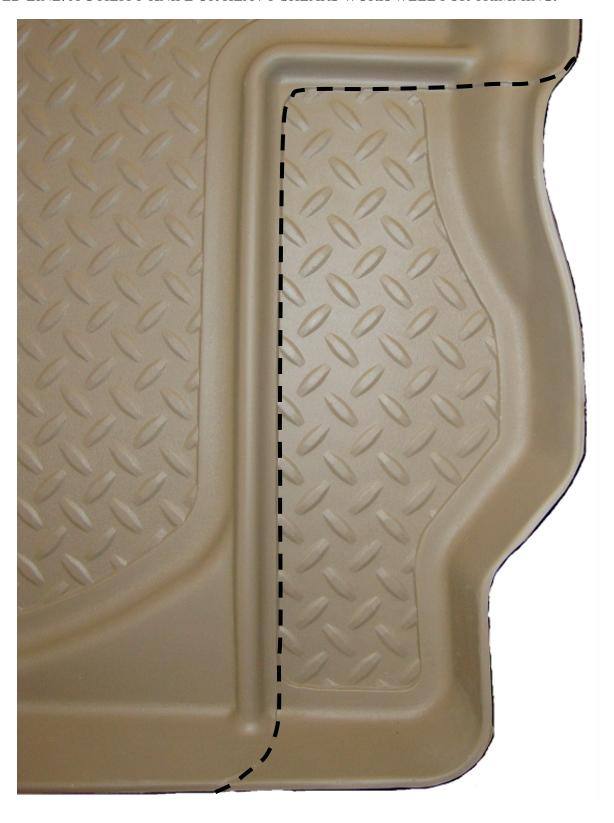
PHOTO SHOWING TRIMMED LINER INSTALLED IN A WRANGLER UNLIMITED WITH THE OPTIONAL FACTORY SUB-WOOFER.
