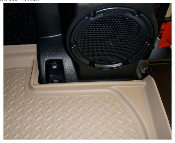
LINER SHOWN TRIMMED TO ACCESS THE CARGO TIE-DOWN HOOKS AND ALSO TO ACCESS THE FACTORY CHILD SAFETY SEAT "LATCH" LOCATIONS ALONG THE FRONT WALL OF THE LINER. TO ACCESS THE LATCH AREAS, REMOVE THE MATERIAL FROM THE LOWERED AREAS.
