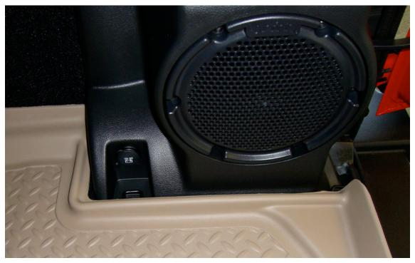
LINER SHOWN TRIMMED TO ACCESS THE CARGO TIE-DOWN HOOK LOCATIONS AND ALSO TO ALLOW INSTALLATION OF  $2^{\rm ND}$  ROW SEAT ON TOP OF LINER.
