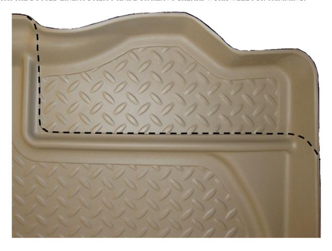
CARGO LINER TRIMMED AND INSTALLED IN A WRANGLER WITH THE FACTORY SUB-WOOFER.
