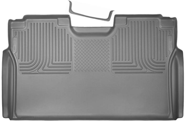
TO EASE INSTALLATION OF YOUR NEW SUPERCREW LINER, MOVE BOTH FRONT SEATS TO THEIR MOST REARWARD POSITION. ONCE LINER IS INSTALLED, REPOSITION THE SEATS AS DESIRED. IF YOUR TRUCK IS EQUIPPED WITH A 40/20/40 SPLIT BENCH FRONT SEAT, YOU WILL NEED TO TRIM YOUR LINER TO ACHIEVE THE PROPER FIT. SEE IMAGE ON BACK FOR TRIMMING DETAILS. TRIM LINER LEAVING AN APPROXIMATE ¼" LIP AROUND THE CUPHOLDER PROFILE AS SHOWN IN THE IMAGES BELOW. A UTILITY KNIFE OR HEAVY SHEARS WORK WELL FOR TRIMMING.
