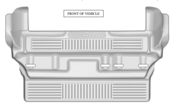
BEFORE ATTEMPTING TO INSTALL YOUR LINER, FIRST FLIP/FOLD YOUR SECOND ROW BENCH SEATS FORWARD TO EXPOSE THE  $3^{\rm RD}$  ROW FLOOR PAN. WITH THIS DONE YOU CAN POSITION THE LINER IN THE FLOOR ORIENTED AS SHOWN ABOVE.
