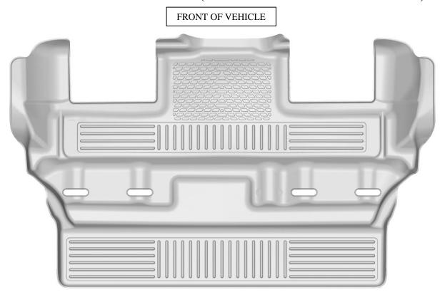
BEFORE ATTEMPTING TO INSTALL YOUR LINER, FIRST FLIP/FOLD YOUR SECOND ROW BUCKET SEATS FORWARD TO EXPOSE THE  $3^{\rm RD}$  ROW FLOOR PAN. WITH THIS DONE YOU CAN POSITION THE LINER IN THE FLOOR ORIENTED AS SHOWN ABOVE. THE "TONGUE" AREA PROVIDES COVERAGE BETWEEN THE  $2^{\rm ND}$  ROW BUCKET SEATS AND TUCKS UNDER THE REAR EDGE OF YOUR  $2^{\rm ND}$  SEAT LINER.
