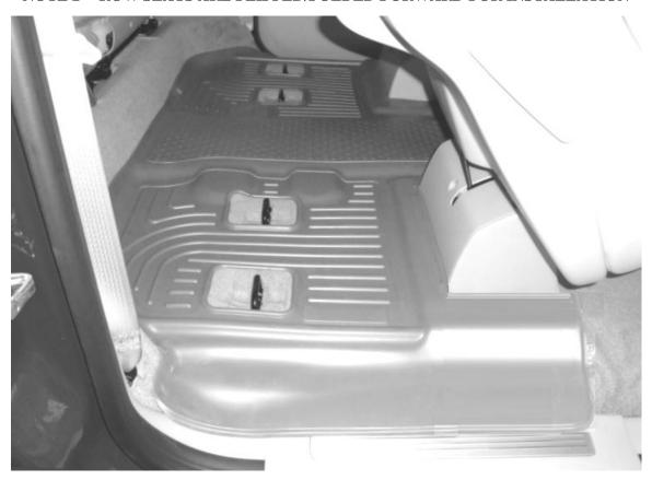
NOTE SEAT ATTACHES TO FLOOR THROUGH LINER
