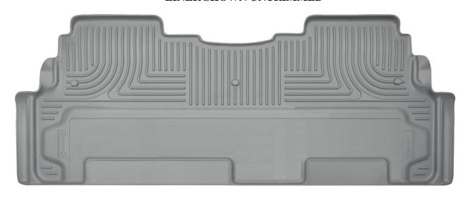
LINER SHOWN TRIMMED TO ACCOMMODATE REPOSITIONING OF  $2^{\rm ND}$  ROW SEATS TO ALLOW MORE  $3^{\rm RD}$  SEAT LEG ROOM
