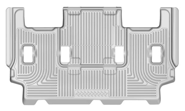
TO EASE INSTALLATION OF YOUR SECOND SEAT LINER, MOVE BOTH FRONT SEATS TO THEIR MOST FORWARD POSITION. THEN, FLIP UP / FOLD FORWARD THE  $2^{\rm ND}$  ROW SEATS TO EXPOSE THE CARPETING UNDER THE SEATS. ONCE LINER IS INSTALLED, FOLD THE  $2^{\rm ND}$  ROW SEATS DOWN WITH THE LEGS PASSING THROUGH THE TRIMMED HOLES IN LINER. TAKE CARE THAT THEY ARE LATCHED SECURELY.LASTLY, REPOSITION THE FRONT SEATS AS DESIRED.
