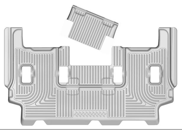
FOR MODELS WITH  $2^{ND}$  ROW BUCKET SEATING THAT INCLUDE A CONSOLE BETWEEN THE  $2^{ND}$  ROW SEATS, USE THE MOLDED IN TRIM STEP TO TRIM AS SHOWN ABOVE.
