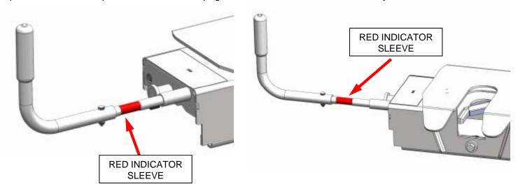
There is another visual aid that indicates if the hitch head is closed and locked. This is shown in the picture below with a green shaft that protrudes from the side of the hitch head. If the king pin has been correctly installed into the mouth of the hitch head the slide bar will close, the red indicating sleeve will disappear and the green indicator pin will protrude out as shown below. Cross member, uprights and base rails removed for clarity.
