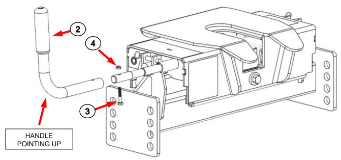
6. Use a wrench to trip the lock mechanism to close the hitch head. Be careful to keep your body away from any moving parts. The handle should rotate and point down towards the bed of the pickup truck.
