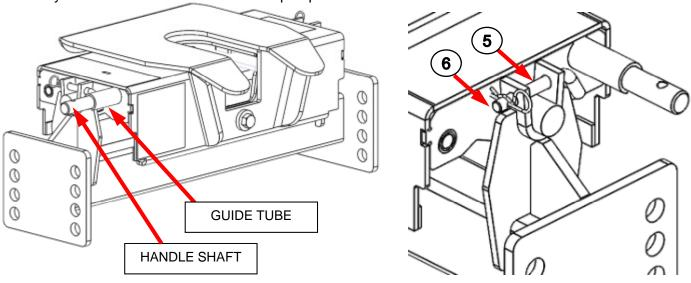
4. Hold the handle with the grip pointed upward and slide the handle (2) onto the handle shaft.
