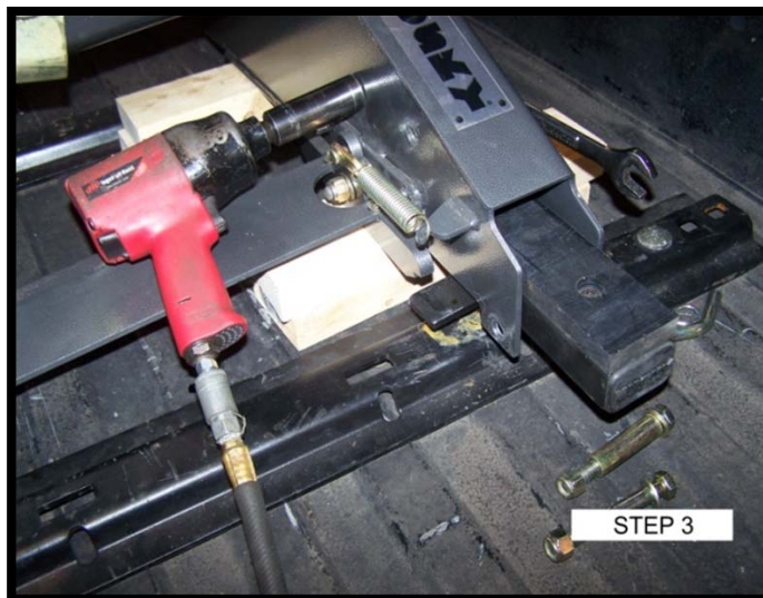
Remove (5) \frac{1}{2} " housing bolts and discard.
