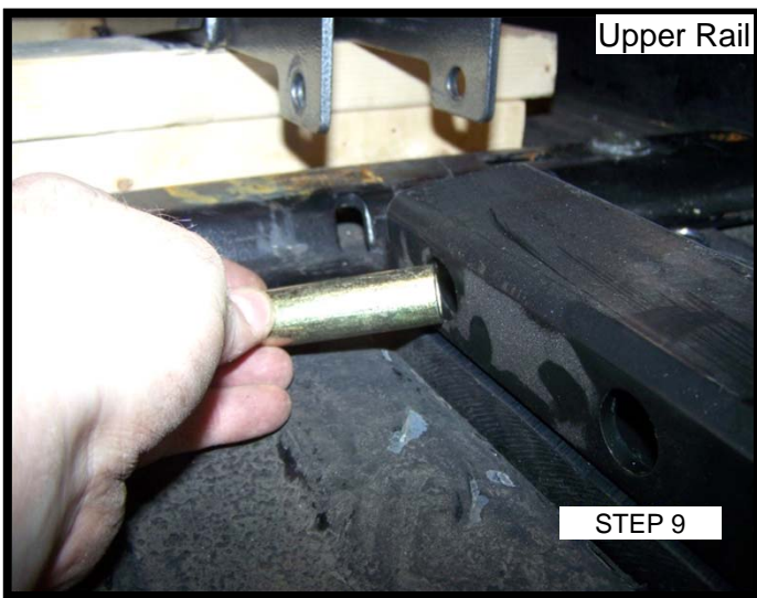
Insert new bushings into holes in upper rail.
