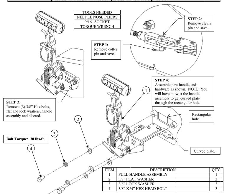
**IMPORTANT!** Check the operation of the flipper plates after new handle is assembled to ensure proper contact with the stop tabs is made. Make adjustments per the 26K Husky-10 instructions if necessary.
