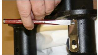
2. Once the drive screw's head is removed; remove the retaining spring. And remove the remainder of the drive screw with the 1/8" drift punch and hammer.
