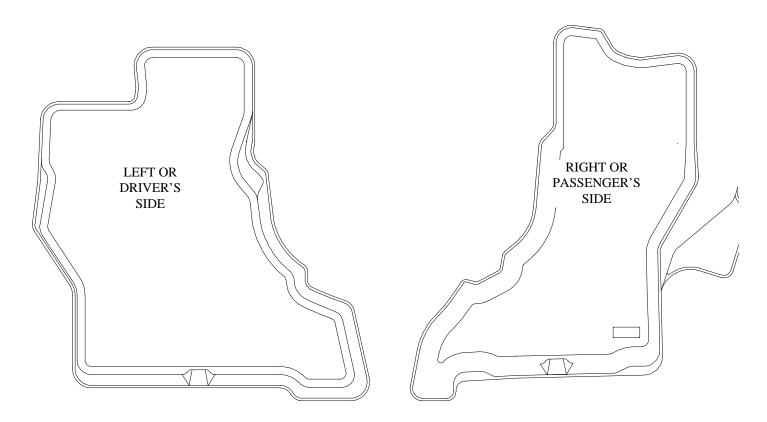
NOTICE: WHEN INSTALLING YOUR PASSENGER SIDE LINER, YOU MAY NOTICE THAT IT DOES NOT MATCH WITH THE EXISTING INNER STEP. THIS IS DUE TO VARIATIONS IN VANS AND VAN CONVERTERS AND CAN BE EASILY REMEDIED. TRIM OFF THE EXCESS PORTION OF YOUR LINER BY TRIMMING ALONG THE TOP OF THE RAISED RIDGE AS SHOWN ABOVE. A UTILITY KNIFE OR HEAVY SCISSORS WORK WELL FOR TRIMMING.
