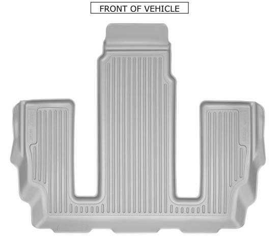
TO EASE INSTALLATION OF YOUR 3<sup>RD</sup> SEAT FLOOR LINER, FLIP BOTH 2<sup>ND</sup> ROW SEATS FORWARD TO ALLOW EASIER ACCESS TO THE 3<sup>RD</sup> ROW FLOOR PAN. ONCE YOU HAVE INSTALLED YOUR LINER, REPOSITION THE 2<sup>ND</sup> ROW SEATS AS DESIRED. NOTE THAT THE "TONGUE" SECTION OF THE 3<sup>RD</sup> SEAT LINER TUCKS UNDER THE BACK EDGE OF THE 2<sup>ND</sup> SEAT LINER
