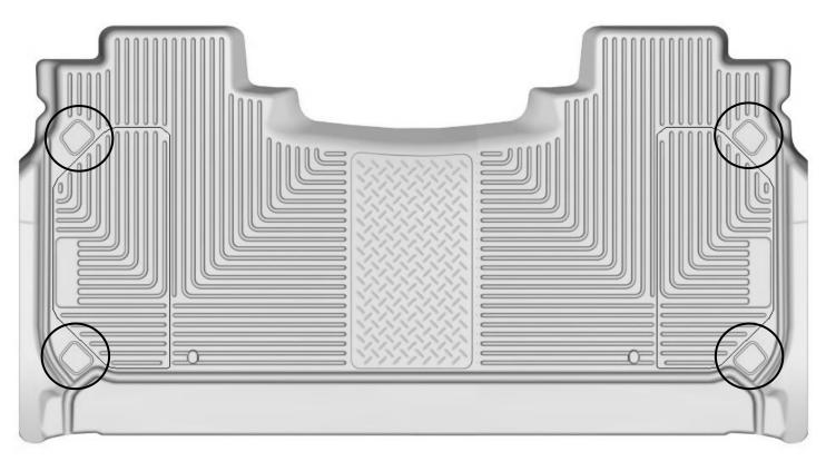
PRIOR TO INSTALLING YOUR 2<sup>nd</sup> SEAT LINER, SLIDE BOTH FRONT ROW SEATS COMPLETELY FORWARD. WITH THIS DONE, INSTALL THE LINER, POSITIONING IT AS SHOWN ABOVE. ONCE THE LINER IS IN PLACE, REPOSITION THE FRONT SEATS AS DESIRED.
