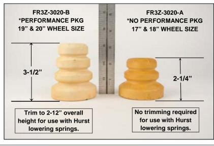
FR3Z-3020-B Trimming Details: These stops need to have the material removed from the small diameter end. It is convenient in that there is physical geometry on the stop which you can use a reference for trimming - trim the stop at the outer edge of the last groove towards the small diameter end. Cutting here will yield an overall height roughly 2-1/2". Install to the strut, and assemble to factory specifications.
