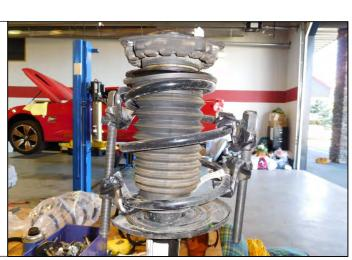
25. Once the upper cup no longer has tension from the spring, remove the nut holding the upper cup in position. A strap wrench may be needed to hold the shaft of the shock to allow the locking nut to be removed.
