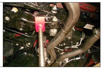
4. Remove the lower bolt from the rear shock.
