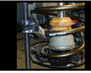
30. Also note that the upper cup assembly has no special alignment for the top of the spring. The upper cup assembly can be installed without any alignment marks.
