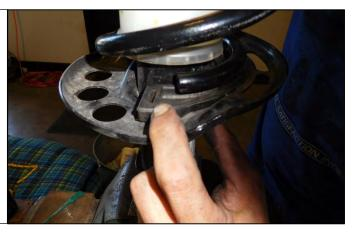
29. To ensure proper spring installation, make sure the Hurst logo is facing up like the image shown.
