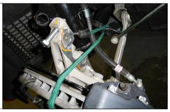
22. Support the strut assembly and remove the three strut tower bolts loosened in the previous step, then remove the strut assembly. Pay close attention to brake and ABS lines when removing the strut assembly, making sure not to snag them.
