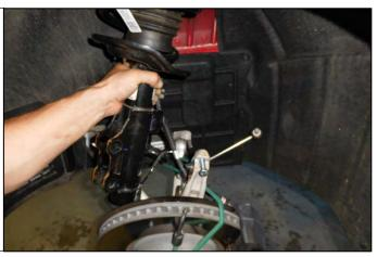
23. Remove the rubber cap from the top of the strut, exposing the nut. The nut will be removed in a later step.
