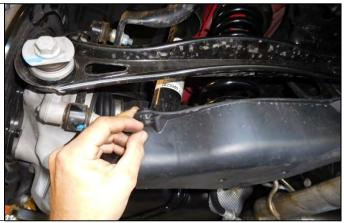
3. Support the rear control arm with a screw jack or Hydraulic jack.
