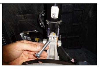
16. Remove the bracket bolt for the rubber brake line. Unclip retainer for the ABS sensor wire. Ensure both are free from the strut and don't have any tension on them.
