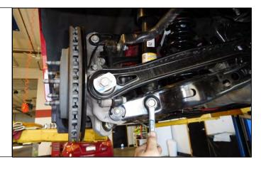
5. Loosen the bolt that connects the hub assembly to the rear lower control arm.
