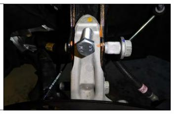
20. Loosen but do not remove the three upper strut assembly bolts from the strut tower.
