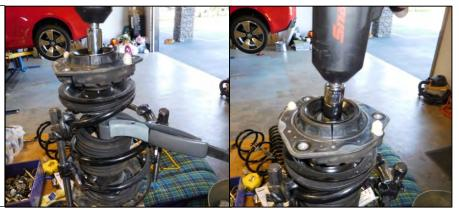
26. Remove the upper cup and rubber boot before removing the spring.
