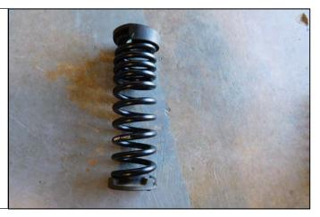
11. Install the factory upper and lower rubber on the new Hurst lowering spring. Align the spring stops on the top and bottom. To ensure proper installation, make sure the Hurst logo is facing up.
