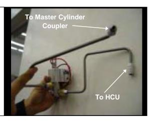
5. Remove left Master Cylinder nut from Master Cylinder.
