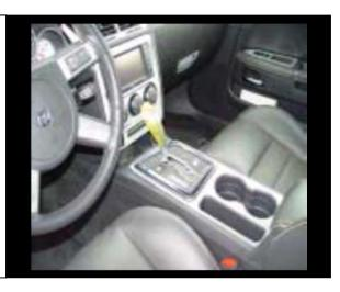
12. Reconnect the battery and turn ignition switch to the "ON" position. While still in park and NOT depressing your brake pedal, activate and engage your Hurst Roll/Control system (make sure you can hear the clicking of the solenoid) several times and check fuse. If fuse is burned, check all electrical connections for a short and correct any problems immediately.
