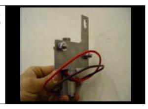
3. Tighten the provided adapters and plugs to solenoid as shown.
