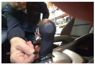
2. Remove screw cover from front of factory shifter.
