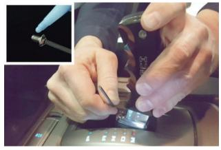
5. Apply loctite to **screw (2)** then install it into front of shifter handle.
