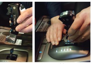
4. Install assembled shifter handle (1).
