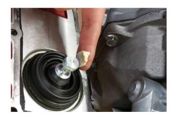
8. Apply a small amount of white lithium grease to the socket in the transmission. Again, if this is a new transmission you can wipe some off the stock shifter and use this.
