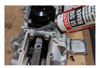
12. Install rear cover and bolt in place suing supplied hardware.
