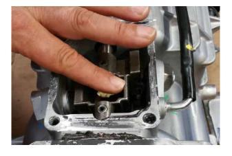
9. Apply a bead of RTV to Seal shifter flange before mounting.
