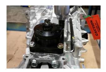
11. Apply a bead of RTV to rear cover flange.
