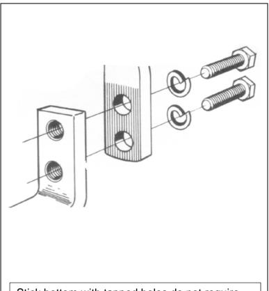
Stick bottom with tapped holes do not require stiffener plate.
