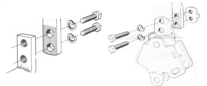
Stick bottom with tapped holes do not require stiffener plate.
