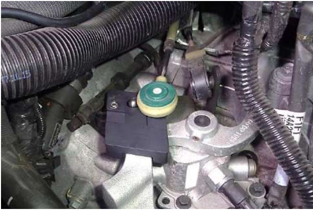
43. Snap the cable end onto the ball stud.
