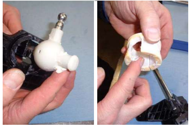
34. Temporarily transfer any grease from the main and side pivot balls into the main pivot cup (to be used later).
