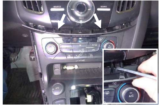
16. Tilt the bezel downward, and locate the two clips toward the rear. With a small, flat-tip screwdriver, release each clip to further separate the bezel from the panel.
