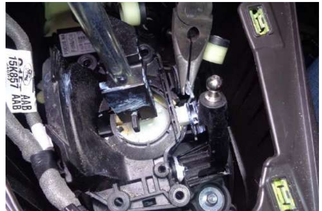
29. Use pliers to lift the top leg of the centering spring up off the rubber grommet on the side shaft.
