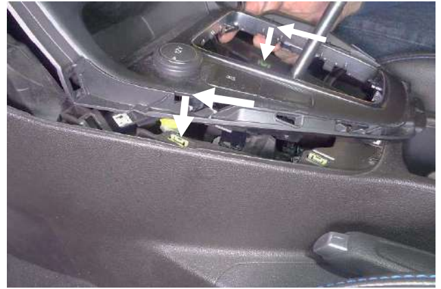
59. Install the power panel with a “forward-then-down” motion (the reverse of Steps 20 and 19). First move the panel forward, inserting its alignment tabs in their slots in the center dash. Then push it downward, snapping it into the 4 clips in the center console.
