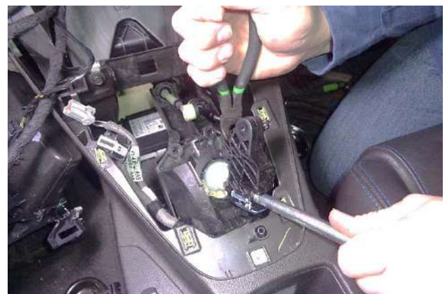
30. While holding the spring open, remove the shift lever and shifter top housing from the bottom housing.
