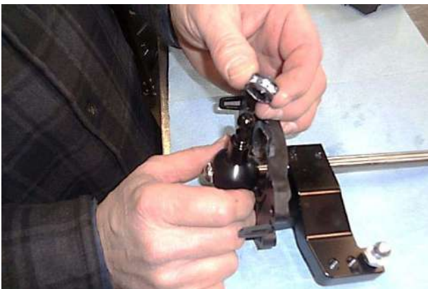
45. Push the centering spring grommet onto the side shaft.
