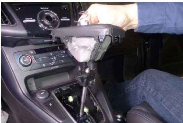
64. Slip the assembled boot and reverse lockout sleeve onto the shift lever. • To install the Hurst shift knob, continue with Step 65 below. • To reinstall the stock shift knob, go to Step 73.
