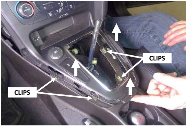
19. Lift the bottom of the panel up just far enough to release it from its 4 clips.
