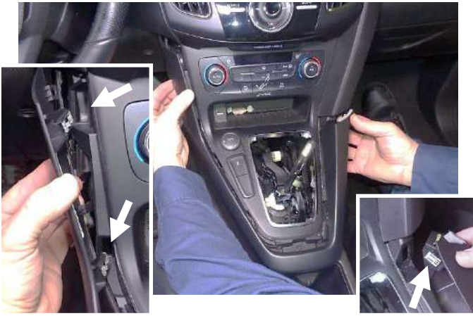
62. Reinstall the shift console trim, taking care to engage the 2 clips on the left, and the 1 clip on the right.
