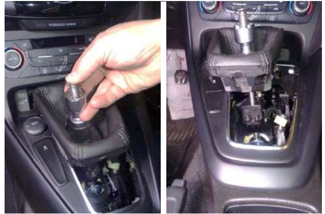
65. Move the shift lever into REVERSE gear.
