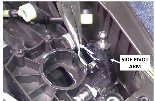
48. Use pliers to lift the top leg of the centering spring far enough to allow insertion of the side shaft into the side pivot arm.
