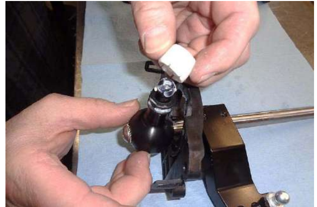
46. Apply grease to side pivot ball, then snap the side pivot cup onto the ball. NOTE: Where grease is required during assembly, first use the grease that was transferred to the main pivot cup at Step 34. Then use new white lithium grease, if required.
