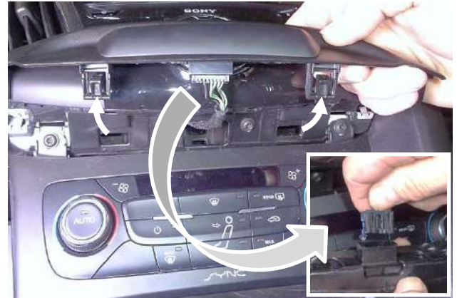
17. Tilt the bezel upward, disconnect the electrical plug on the back, and remove the bezel from the vehicle.
