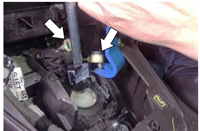
24. Carefully pry the 2 shifter cable ends off of their ball studs.
