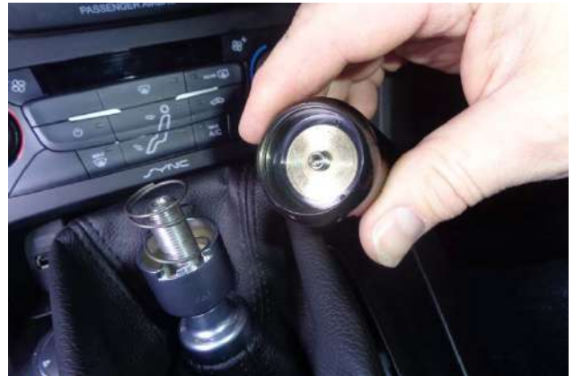
66. Install the set screw (3) in the shift knob (4), leaving 2-3 threads exposed.
