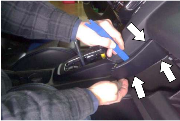
13. Open the glove box, then use a trim removal tool to remove the small console side panel just below the passenger-side dash board. (You may close the glove box after removing the panel.)
