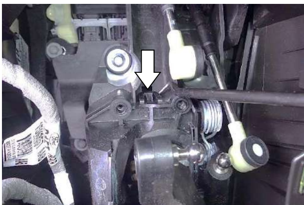
27. With a cotter key extractor or bent pick, release the clip at the front of the shifter assembly.
