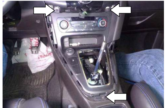
60. Install and tighten the 3 power panel screws.
