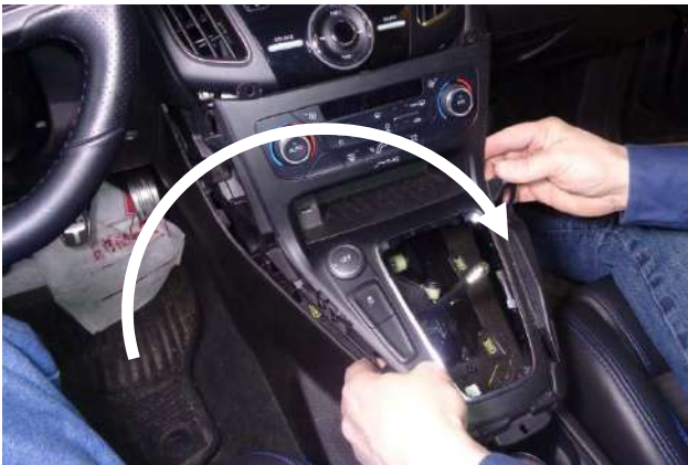
57. Carefully flip the power panel back over the center console.
