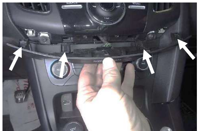
61. Reconnect the center panel bezel plug. Then line up the 4 clips on the bezel with their slots on the panel and reinstall the bezel.
