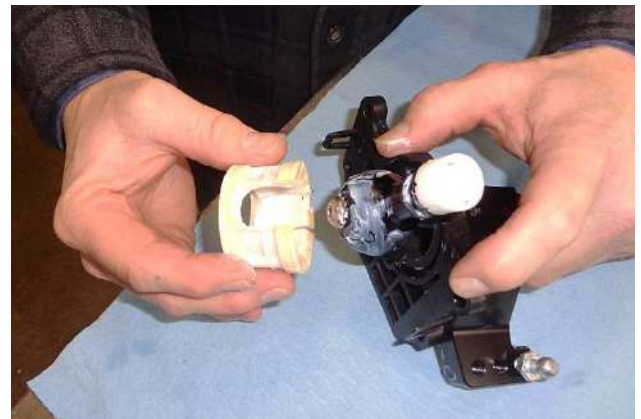
47. Apply grease to main pivot ball, then snap the main pivot cup onto the ball.
