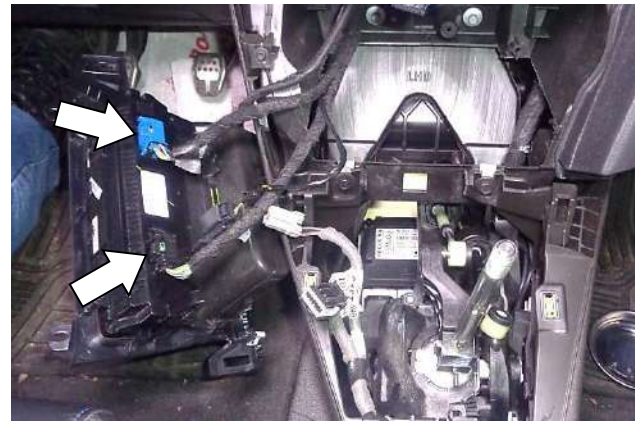
23. Disconnect the blue (AUTO) and black (AC) connectors, and remove the power panel from the vehicle.
