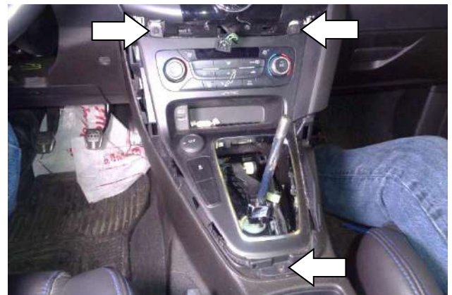
18. Remove the 3 power panel screws.
