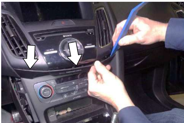
15. Use a trim tool to start separating the bezel from the center panel.
